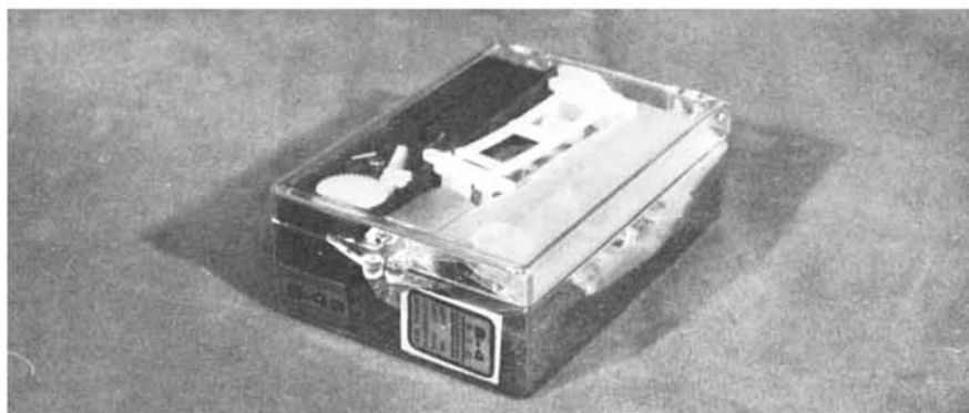
The receiver and decoder, completed and ready for tuning, then installation into their cubical type case.
